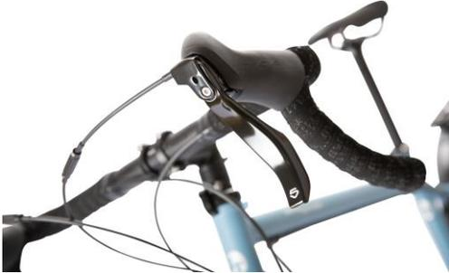
Riding a drop bar with a fully integrated brake-/shift lever and using it with a Rohloff Speedhub hub is what many riders have dreamed of. The revised interior of the Shift:R II is being used for the Shift:R Road and combined with the excellent braking performance of the TRP Hylex disc brake.
