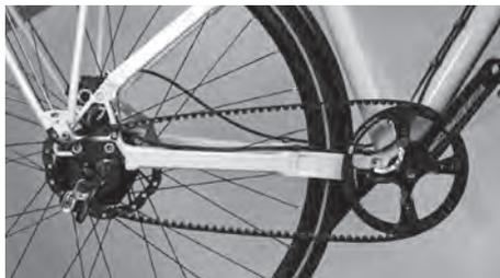
Minimize the distance between the axle of the bottom bracket and the rear axle so that the belt can be fitted to the front sprocket without tension. The tools required to reduce the distance may vary depending upon manufacturer. Always follow the instructions of the particular
