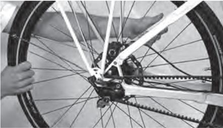
5. Rotate the cranks 10-15 times and check the alignment of the belt. The belt should slightly touch, or come just short of touching the inside flange of the rear sprocket (within 1mm). A constant distance of 0.5mm between belt and flange is recommended.
