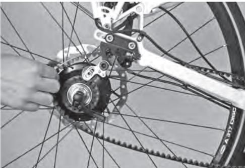
3. Place the belt on the rear sprocket and mount the rear wheel into the rear dropouts.
