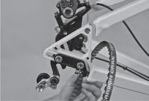
1. Open the frame break or 'gate' on the frame's rear triangle. Since this break may vary from one manufacturer to another, you'll need to follow the instructions of the manufacturer of your frame. In the following illustrations the frame is opened at the dropout. Insert the belt through the opening of the frame.
