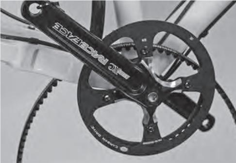
2. Hang the belt over the bottom bracket and lock the frame gate.
